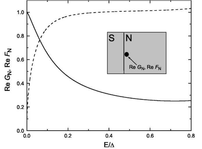
FIG. 2. Calculated density of states ( $\text{Re } G_N$ , dashed line) and pair amplitude ( $\text{Re } F_N$ , solid line) as induced by a superconductor into a normal metal, with  $\gamma_B = 5$ ,  $\gamma = 0.1$ , and  $d_N \gg \xi_N$ . The functions are plotted for the  $N$  side of the interface, as indicated.
