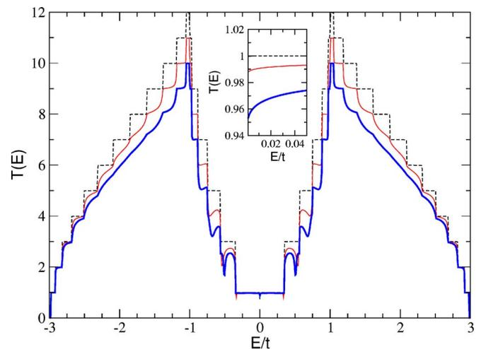
FIG. 4. (Color online) Dashed (black) line: transmission spectrum for ribbons with  $N=24$  atoms in the ideal case. Thin (red) line: removing one atom from the edge. Thick (blue) line: removing two atoms on the top and bottom edges. Inset: Detail of the transmission in the low energy sector. The effect of removing one or two atoms on the border is very small in the lowest conductance plateau.
