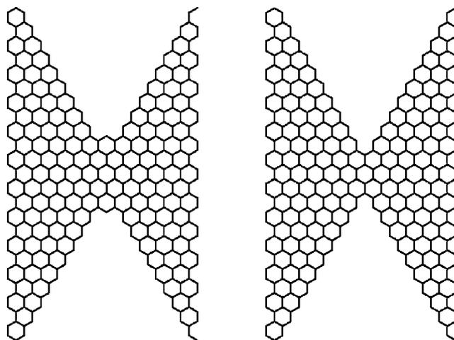
FIG. 7. Schematic atomic structure of wedge-shaped constrictions.
