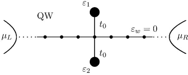
FIG. 1. Scheme of side-coupled quantum dots attached laterally to a perfect quantum wire (QW). The QW is coupled to the left (L) and right (R) noninteracting leads.
