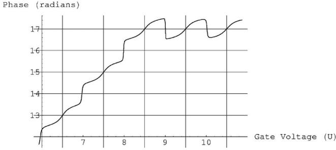
FIG. 3. The phase of the transmission amplitude for the parameters given by Eq. (12). A small section of the previous phase figure is enlarged in order to allow one to follow the details more closely. The perpendicular grid lines are located at resonances.
