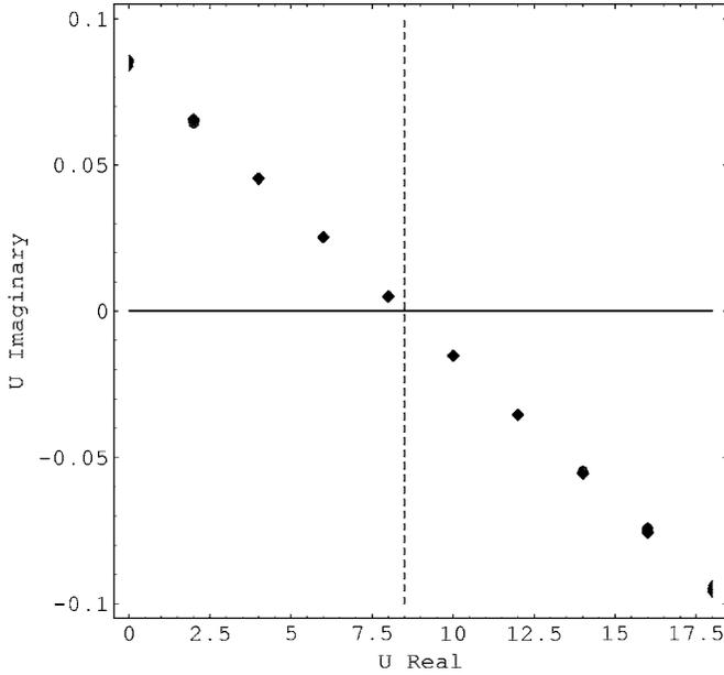
FIG. 4. Zeros of  $t^{QD}(U)$  [see Eq. (22) below] with parameter values  $A=1$ ,  $B=2.5$ ,  $U_c=8.5$ ,  $\gamma=0.01$ .
