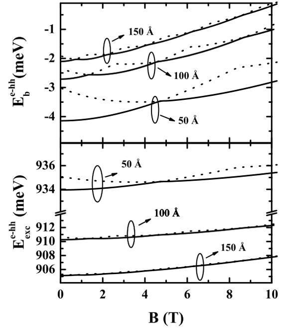
FIG. 5. Binding energies (top) and total exciton energies (bottom) of  $e$ - $hh$  excitons in Si/Si<sub>0.70</sub>Ge<sub>0.30</sub> type-II QWR as a function of the magnetic field for 50, 100, and 150 Å wire radii, with abrupt interfaces. Solid lines are related to ground state excitons, while dotted lines are first excited states.
