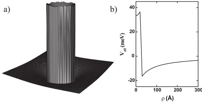
FIG. 3. (a) Effective Coulomb potential for electrons in a type-II Si/Si<sub>1-x</sub>Ge<sub>x</sub> QWR with 50 Å wire radius. (b) The plot of this potential as a function of  $\rho$ , showing a depression near the interface between materials.
