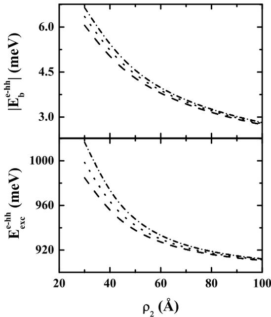
FIG. 4. Binding energy (top) and ground state energy (bottom) of  $e$ - $hh$  excitons in Si/Si<sub>0.70</sub>Ge<sub>0.30</sub> type-II QWR as a function of the wire radius, for interfaces thicknesses  $w$  of 0 Å (solid), 5 Å (dashed), 10 Å (dotted), and 15 Å (dashed-dotted).
