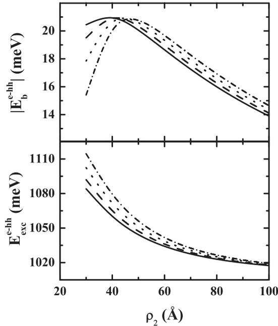
FIG. 1. Binding energy (top) and ground state energy (bottom) of  $e$ - $hh$  excitons in  $\text{Si}/\text{Si}_{0.85}\text{Ge}_{0.15}$  type-I QWR as a function of the wire radius, for interface thicknesses  $w$  of 0 Å (solid), 5 Å (dashed), 10 Å (dotted), and 15 Å (dashed-dotted).
