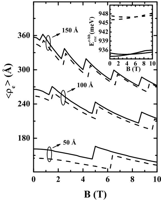
FIG. 6. Average radius of the electron ground state in Si/Si<sub>0.70</sub>Ge<sub>0.30</sub> type-II QWR as a function of the magnetic field, for 50, 100, and 150 Å wire radii, considering  $w=0$  Å (solid) and  $w=15$  Å (dashed). Inset: Exciton energy dependence with the applied magnetic field, for the ground and first excited states of a 50 Å QWR radius with  $w=0$  Å (solid) and  $w=15$  Å (dashed).
