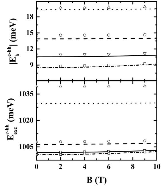
FIG. 2. Binding (top) and ground state exciton energies (bottom) of  $e$ - $hh$  pairs in  $\text{Si}/\text{Si}_{0.85}\text{Ge}_{0.15}$  type-I quantum wires as functions of magnetic field, with  $w=0$  Å (lines) and  $w=15$  Å (symbols), for several values of wire radius  $\rho_2$ : 50 Å (dotted,  $\triangle$ ), 100 Å (dashed,  $\circ$ ), 150 Å (solid,  $\nabla$ ), and 200 Å (dashed-dotted,  $\square$ ).
