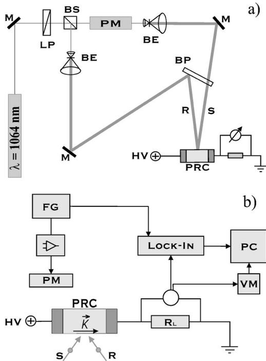
FIG. 1. (a) Experimental setup (schematically). LP, combination of a half-wave plate and a polarizer; BS, beam splitter; BP, beam splitting plate; PM, phase modulator; BE, beam expander; M, mirror; PRC, the studied crystal. A YAG:Nd laser at  $\lambda = 1064$  nm was used. (b) Diagram demonstrating the electronic detection of SCW. HV, high-voltage source; RL, loading resistor; FG, function generator; VM, voltmeter for dc measurements.
