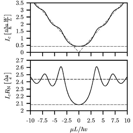
FIG. 2. Critical current  $I_c$  and  $I_c R_N$  product of a ballistic Josephson junction (length  $L$  short compared to the width  $W$  and superconducting coherence length  $\xi$ ), as a function of the Fermi energy  $\mu$  in the normal region. The asymptotes (21) and (22) are indicated by dashed lines.
