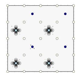
FIG. 11. (Color online) Charge density plot of the charge ordered state localized in the TiO<sub>2</sub> layer of the *n*-type interface. Ti<sup>3+</sup> with an occupied  $d_{xy}$  orbital and Ti<sup>4+</sup> marked by light and dark blue (gray) circles, respectively, are ordered in a (45°) checkerboard manner. Oxygens are marked by white circles. The plotted area corresponds to four  $c(2 \times 2)$ -simulation cells.
