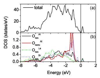
FIG. 7. (Color online) Density of states of the interface with an oxygen vacancy in the  $AlO_2$  layer: (a) total; (b) projected DOS of the O 2p states of the oxygens surrounding the vacancy. Most of the density of the unoccupied gap state lies in the vacancy (see the text).
