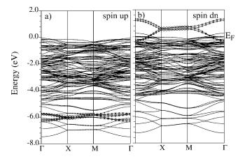
FIG. 4. Spin resolved LDA+U band structure of the oxygen states in the *p*-type LaAlO<sub>3</sub>-SrTiO<sub>3</sub> interface with FM order of the oxygen holes. States localized near one of the magnetic oxygen ions in the AlO<sub>2</sub> layer of predominantly  $P_{\pi}$  hole character (see text) are emphasized with circles; these correspond to (a) lower (majority) and (b) upper (minority) Hubbard bands.
