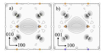
FIG. 8. (Color online) Charge density distribution of the unoccupied O 2p states around an oxygen vacancy in the AlO<sub>2</sub> layer. (a) and (b) show a cut through the xy and xz planes, respectively, with the vacancy positioned at (0.5, 0.5). The positions of O, Al, and Ti ions are marked by white, orange (gray), and blue (dark gray) circles, respectively.
