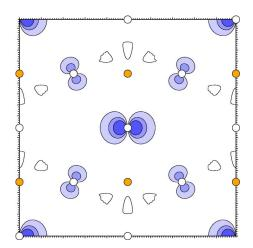
FIG. 3. (Color online) Charge density plot of the ferromagnetically coupled oxygen holes localized in the AlO<sub>2</sub> layer, illustrating the  $P_{\pi}$  hole state centered around  $O_{Al}^*$  at (0.0,0.0) and (0.5,0.5). The figure contains the simulated  $p(2 \times 2)$  supercell, the positions of O and Al atoms are marked by white and orange (gray) circles, respectively.
