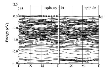
FIG. 6. Spin resolved band structure of the oxygen states in the *p*-type LaAlO<sub>3</sub>-SrTiO<sub>3</sub> interface with AFM order of the oxygen holes. States localized near one of the magnetic oxygen ions in the AlO<sub>2</sub> layer of predominantly  $P_{\pi}$  hole character (see text) are emphasized with circles; these correspond to (a) upper (majority) and (b) lower (minority) Hubbard bands.
