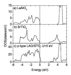
FIG. 2. LDA density of states of (a) bulk LaAlO<sub>3</sub>, (b) bulk SrTiO<sub>3</sub>, and (c) the *p*-type LaAlO<sub>3</sub>-SrTiO<sub>3</sub> interface in GGA. The bulk DOS are obtained for the experimental lattice constants of the respective materials.
