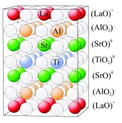
FIG. 1. (Color online) Schematic picture of the *p*-type  $(AlO_2)^-/(SrO_2)^0$  interface, in the smallest cell with two oppositely oriented  $(SrO)^0$ - $(AlO_2)^-$  interfaces. White unlabeled circles denote the oxygen ions.
