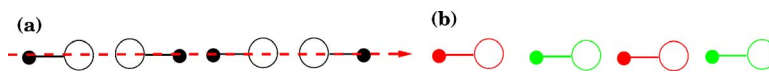
FIG. 6. (Color online) Schematic of dimers flipping after a single scan above a row of alternating dimers of an original c(4 \times 2) structure shown in (a). Low temperatures and large frequency shifts are assumed. The red dashed line indicates the scan direction. In (b), dimers that changed their direction once are shown in green, while those that changed their directions twice in red. At the end of the scan, red dimers remain in their original state, whereas green dimers flipped. Lower and upper dimer atoms are shown with the small black and large open circles, respectively.
