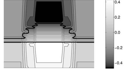
FIG. 3. Contour plot of the electrostatic potential energy  $V_p$ . A slice in the  $x$ - $z$  plane through the center of the QD is depicted. The result is shown for the smallest QD but is qualitatively the same for all the investigated QD sizes.
