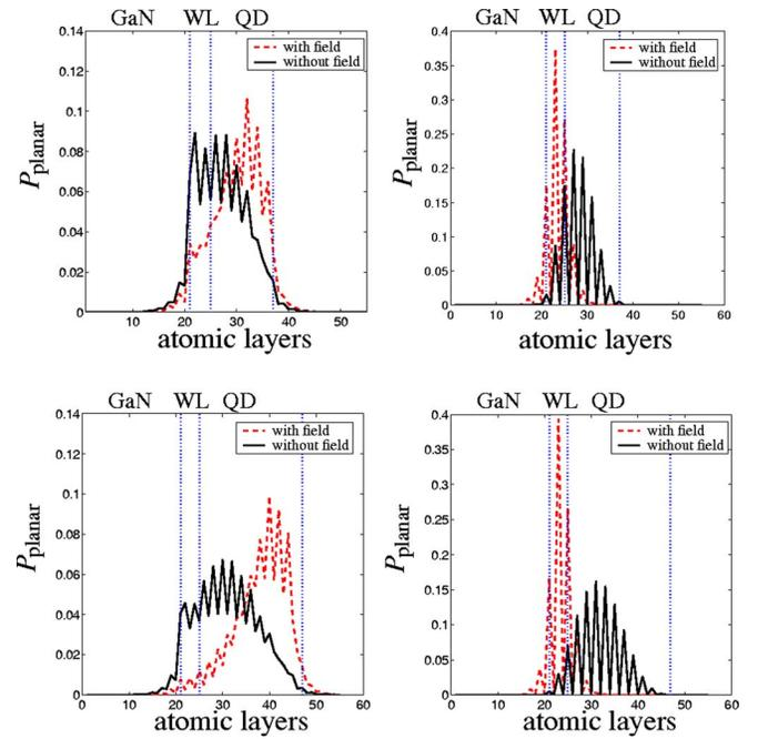
FIG. 5. (Color online) Planar-integrated probability density  $P_{\text{planar}}$  for the electron (left) and the hole (right) ground state, without (solid lines) and with (dashed lines) built-in field for the smallest (top) and the largest (bottom) QD.
