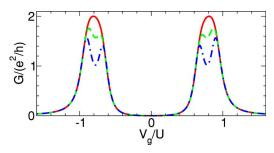
FIG. 13. (Color online) Gate voltage dependence of the total conductance G for the parameters of Fig. 10 and different magnetic fields  $\mathcal{H}=0$  (solid line), and  $\mathcal{H}=0.065\Gamma=0.5T_K$  (dashed line), and  $\mathcal{H}=0.13\Gamma=T_K$  (dashed-dotted line).
