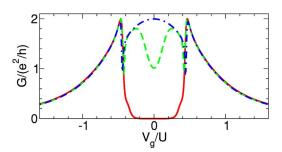
FIG. 14. (Color online) Gate voltage dependence of the total conductance G for the parameters of Fig. 11 and different magnetic fields  $\mathcal{H}=0$  (solid line),  $\mathcal{H}=0.003\Gamma=T^0=0.0026T_K^0$  (dashed line), and  $\mathcal{H}=0.03\Gamma=10T^0=0.026T_K^0$  (dashed-dotted line).
