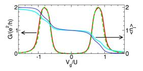
FIG. 10. (Color online) Gate voltage dependence of the total conductance G and total occupancies  $\langle n_j \rangle$  of a spin-degenerate side-coupled double-dot system [see Fig. 1(D)] with  $U/\Gamma=8$  and  $t_{1,2}/\Gamma=4$ . Solid line with left y-axis: NRG data for G from Ref. 28. Dashed line with left y-axis: fRG approximation of G with flow of vertex. Thick solid line with right g-axis: fRG approximation of g-axis: fRG approximati
