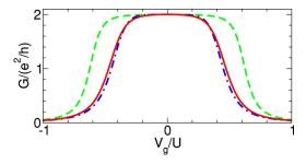
FIG. 3. (Color online) Gate voltage dependence of the linear conductance for the same parameters as in Fig. 2. Solid line: Exact Bethe ansatz solution from Ref. 21. Dashed line: fRG approximation without flow of the interaction. Dashed-dotted line: fRG approximation with flow of vertex.
