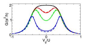
FIG. 4. (Color online) Gate voltage dependence of the total conductance G of a single dot with  $U/\Gamma=3\pi$  and  $\mathcal{H}/\Gamma=0$ , 0.058, 0.116, and 0.58 from top to bottom. In units of the  $V_g=0$  Kondo temperature  $T_K^{\rm NRG}/\Gamma=0.116$  these fields correspond to  $\mathcal{H}=0$ , 0.5 $T_K^{\rm NRG}$ ,  $T_K^{\rm NRG}$ , and  $5T_K^{\rm NRG}$ . Solid line: NRG data from Ref. 66. Dashed line: fRG approximation with flow of vertex.
