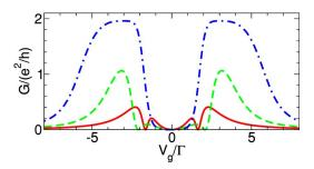
FIG. 18. (Color online) Gate voltage dependence of the total conductance G of a parallel double dot with generic  $\Gamma_j^l$ , s=-1, spin-degenerate levels,  $\delta=0$ , local interaction  $U/\Gamma=4$ , and different nearest-neighbor interactions U'=0 (solid line),  $U'/\Gamma=2$  (dashed line), and  $U'/\Gamma=4$  (dashed-dotted line). The  $\Gamma_j^l$  are as in Fig. 17. Note that here  $V_g$  is shown in units of  $\Gamma$ .
