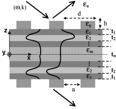
FIG. 1. Geometry of the studied configuration. The structure is invariant along  $(Oy)$  and symmetrical with respect to the  $(Oxy)$  and  $(Oyz)$  planes. The periodicity of the structure and the spatial frequency of the incident wave are chosen in order to excite two independent eigenmodes.
