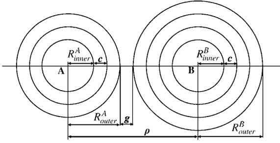
FIG. 1. Schematic drawing of two MWNTs, A and B, with center-to-center distance  $\rho$ , inner radii  $R_{inner}^A$  and  $R_{inner}^B$ , van der Waals gap  $g$ , and a constant interlayer spacing  $c$ . The value of the outer radius is determined by  $R_{outer} = R_{inner} + (n-1) \times c$ .
