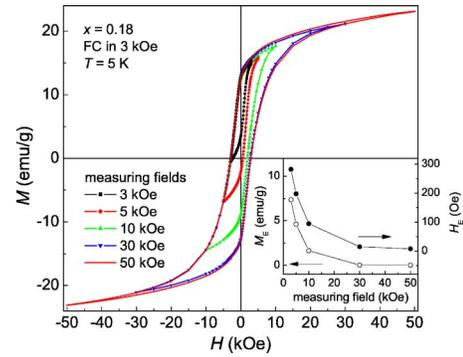
FIG. 7. (Color online) The FC (in 3 kOe) hysteresis loops for  $\text{La}_{0.82}\text{Sr}_{0.18}\text{CoO}_3$  at 5 K with different measuring magnetic fields. Inset: measuring field dependence of  $H_E$  and  $M_E$  at 5 K.
