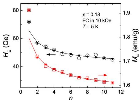
FIG. 5. (Color online) The number of field cycles  $n$  dependence of  $H_E$  and  $M_E$  (open symbols) for  $\text{La}_{0.82}\text{Sr}_{0.18}\text{CoO}_3$  at 5 K after field cooling in 10 kOe. Solid lines show the best fits with Eq. (1) to the data for  $n > 1$ . Solid symbols show the data generated from the recursive sequence (2) as described in the text.
