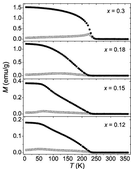
FIG. 2. Temperature dependence of the dc magnetizations with ZFC (open circles) and FC (solid circles) processes for  $\text{La}_{1-x}\text{Sr}_x\text{CoO}_3$  ( $x = 0.12, 0.15, 0.18,$  and  $0.3$ ) samples in 10 Oe.
