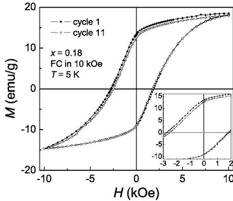
FIG. 4. Training effect of exchange bias in  $\text{La}_{0.82}\text{Sr}_{0.18}\text{CoO}_3$ . Plotted are the first and the eleventh loops at 5 K after field cooling in 10 kOe. Inset: enlarged view of the central region of the loops.
