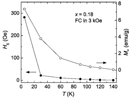
FIG. 6. Temperature dependence of  $H_E$  and  $M_E$  for  $\text{La}_{0.82}\text{Sr}_{0.18}\text{CoO}_3$  after field cooling in 3 kOe.
