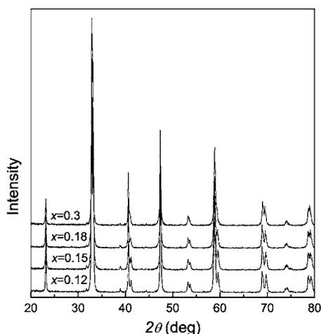
FIG. 1. Powder x-ray diffraction patterns of  $\text{La}_{1-x}\text{Sr}_x\text{CoO}_3$  ( $x = 0.12, 0.15, 0.18,$  and  $0.3$ ) samples at room temperature.
