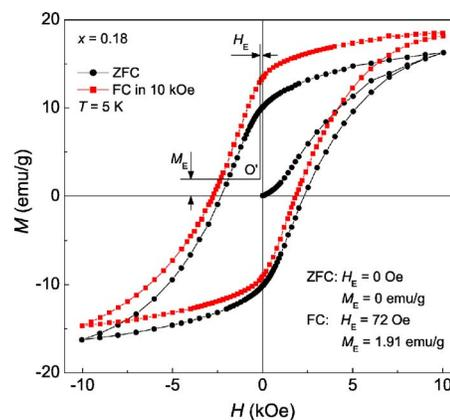
FIG. 3. (Color online) Hysteresis loops of  $\text{La}_{0.82}\text{Sr}_{0.18}\text{CoO}_3$  at 5 K measured after zero-field cooling and field cooling in 10 kOe field.
