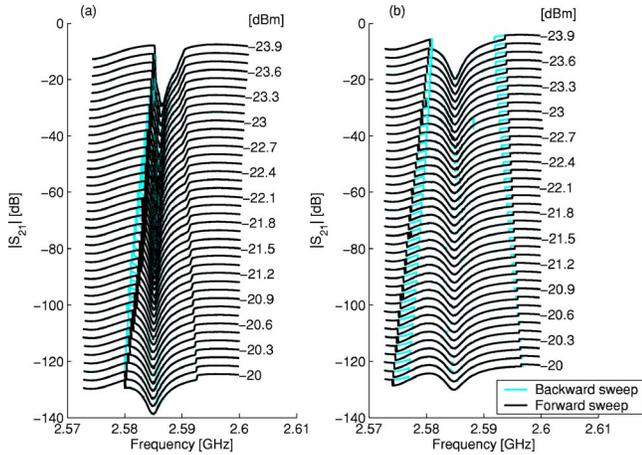
FIG. 4. (Color online). Frequency sweep measurement of the B1 resonator first mode performed in both directions while (a) applying white noise of  $-58$  dBm/Hz (b) without applying external noise. The black line represents a forward sweep, whereas the cyan (gray) line represents a backward sweep. The measured resonance curves were shifted vertically by a constant offset for clarity.
