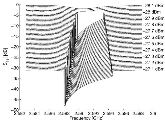
FIG. 2.  $S_{11}$  amplitude measurement of the B1 resonator at its first mode. The measured resonance line shapes are asymmetrical and contain two abrupt jumps at the sides of the resonance. Moreover, the jump frequencies shift outwards as the input power is increased. The measured resonance line shapes were shifted vertically by a constant offset for clarity.
