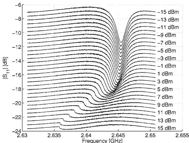
FIG. 8. Duffing oscillator nonlinearity exhibited by a Nb strip-line resonator employing a B2 layout at its first mode. The different plots of the  $S_{11}$  amplitude correspond to different input powers, ranging from  $-15$  dBm to  $15$  dBm in steps of  $1$  dBm. As the input power is increased the resonance becomes asymmetrical and an infinite slope builds up at the left side of the resonance curve. The plots were offset in the vertical direction for clarity.
