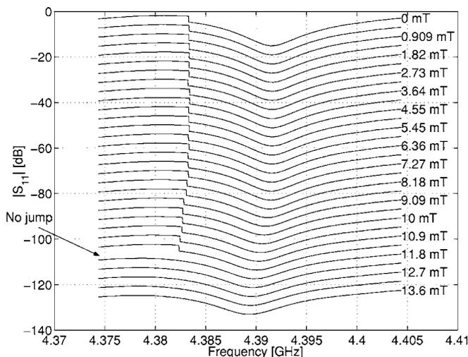
FIG. 7. Increasing the magnetic field gradually from zero while applying a constant input power level of  $-5$  dBm causes the jump in the B2 resonance line shape to disappear at a relatively low value of  $11.8$  mT. This vanishing jump indicates that the jump mechanism is sensitive to the magnetic field. The measured curves were shifted vertically by a constant offset for clarity.
