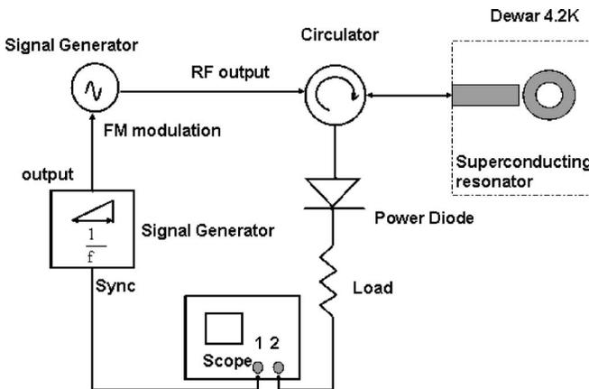
FIG. 10. Frequency sweep time analysis setup. The frequency sweep time of the microwave signal generator was FM modulated by a sawtooth wave form of frequency  $f$ . The reflected power off the resonator was measured by a power diode and an oscilloscope.
