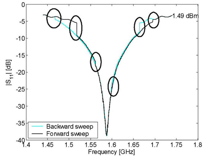
FIG. 5. (Color online).  $S_{11}$  amplitude measurement of the first resonance of the B3 resonator, measured at an input power of 1.49 dBm. The measurement was done using a network analyzer employing 4000 measurement points in each direction. The black line represents a forward frequency scan whereas the cyan (gray) line represents a backward frequency scan. The plot shows clearly three jumps within the resonance line shape in each direction, as indicated by small circles.
