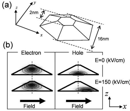
FIG. 2. (a) Schematic of the GaN/AlN dot used for the calculation. (b) Calculated probability density distribution for the ground electron and hole states.
