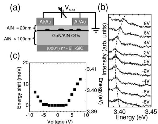
FIG. 1. (a) Schematic of the sample structure used to apply the electric field. (b) Microphotoluminescence spectra for applied voltages between  $-8$  and  $8$  V. (c) Emission energy shift as a function of the applied bias voltage.
