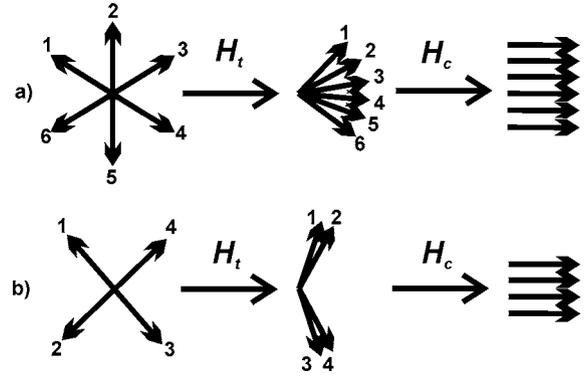
FIG. 1. Sketch of the metamagnetic transitions in helical structures due to an applied external field: (a) screw to fan transition (Refs. 10 and 15); (b) scenario for nearly orthogonal helical structures (Ref. 16). The numbers denote subsequent layers of magnetic atoms.
