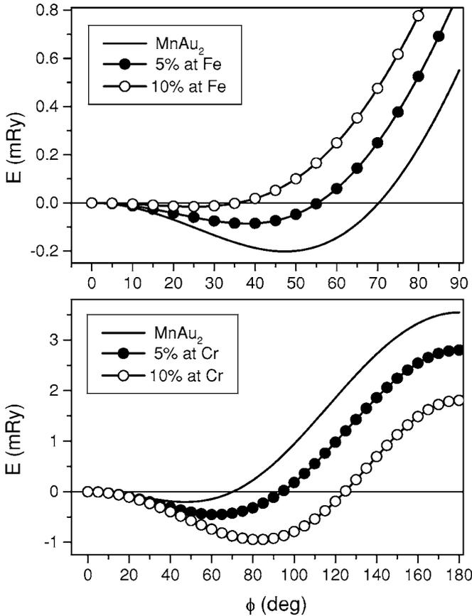
FIG. 2. Calculated energies of the helical structures with respect to the ferromagnetic phase for  $\text{Mn}_{1-x}\text{TM}_x\text{Au}_2$  alloys (TM=Fe,Cr) as a function of the helix angle,  $\varphi$ .
