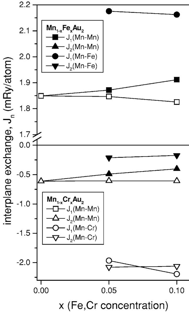
FIG. 3. Partial contributions to the effective interlayer exchange coupling, see Eq. (6), as a function of the concentration of the TM atoms  $x$  in  $\text{Mn}_{1-x}\text{TM}_x\text{Au}_2$  alloys (TM=Fe,Cr).
