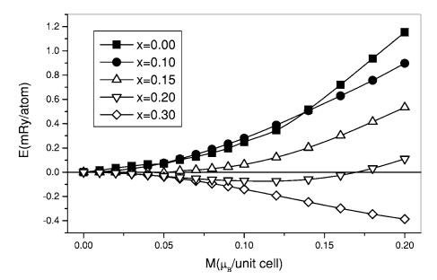
FIG. 3. FSM total energies for  $CoGa_{1-x}Ni_x$  alloys.
