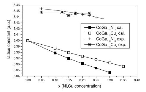
FIG. 1. Calculated (GGA) and experimental (Ref. 24) equilibrium lattice constants of  $CoGa_{1-x}T_x$  alloys.
