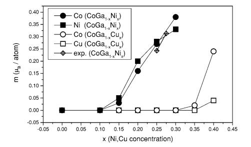
FIG. 2. Calculated groundstate magnetic moments of  $\text{CoGa}_{1-x}T_x$  alloys. Experimental points were subtracted from total magnetization measurements in Ref. 24 and given in  $\mu_B/T$  atom (*T*=Cu, Ni).
