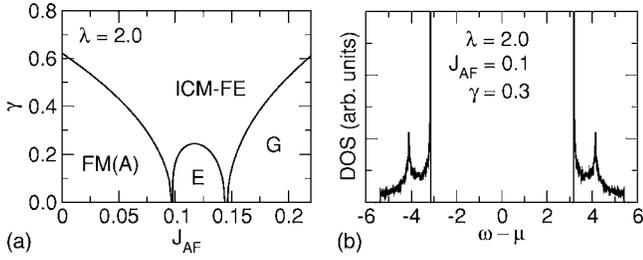
FIG. 4. Results of exact diagonalization of Hamiltonian (10) at  $T=0$  in the thermodynamic limit for  $\lambda=2.0$ ,  $\kappa_1=1$ , and  $\kappa_2=10$ . (a) Ground-state phase diagram and (b) electronic density of states in the ICM-FE phase.
