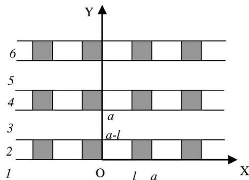
FIG. 1. Birds-eye view of a two-dimensional phononic crystal constructed by rectangular rods (shaded areas) arranged squarely in a uniform host with lattice constant  $a$ ,  $l$  is the distance between two nearest rods. A set of planes parallel to the  $xoz$  plane cuts the system into uniform and composite layers along the  $y$  direction, which are labeled as 1, 3, 5, ... and 2, 4, 6, ..., respectively.
