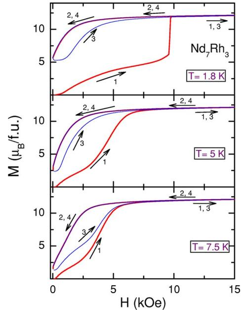
FIG. 2. (Color online) Isothermal magnetization behavior for  $\text{Nd}_7\text{Rh}_3$  (with a VSM) at 1.8, 5 and 7.5 K for the field excursion: 1, 0 to 30 kOe; 2, 30 to 0 kOe; 3, 0 to 30 kOe; 4, 30 to 0 kOe without any break between these paths. Before measurements at each temperature the specimen was zero-field cooled from 50 K.
