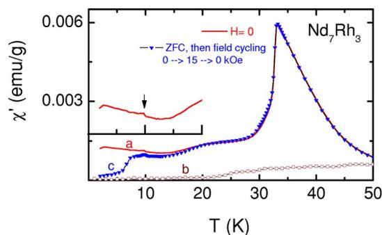
FIG. 5. (Color online) Real part of the ac magnetic susceptibility as a function of temperature for  $\text{Nd}_7\text{Rh}_3$ . The curves *a*, *b*, and *c* are described in the text. To show the presence of a weak feature (marked by vertical arrow), the data below 20 K for curve *a* are also shown in an expanded form. Since the curves for all frequencies overlap, the data for only frequency are plotted.
