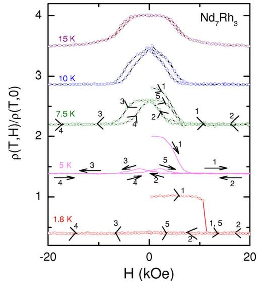
FIG. 4. (Color online) Electrical resistivity (normalized to respective zero-field values in the virgin curve) as a function of magnetic field for  $\text{Nd}_7\text{Rh}_3$ . The paths denoted are the same as described in Fig. 1, though the data are shown in the range –20 to 20 kOe only. The curve for each temperature is shifted along the y axis for the sake of clarity.
