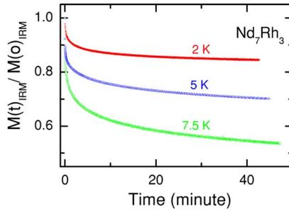
FIG. 3. (Color online) Time ( $t$ ) dependence of isothermal remanent magnetization normalized to the value at  $t=0$  (defined as the time at which  $H$  becomes zero in this measurement) for  $\text{Nd}_7\text{Rh}_3$  (with a VSM) at various temperatures. Before measurements at each temperature the specimen was zero-field cooled from 50 K.
