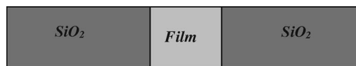
FIG. 10. Profile of two layers of a - (or c -) SiO 2 grains being separated by an interlayer film.
