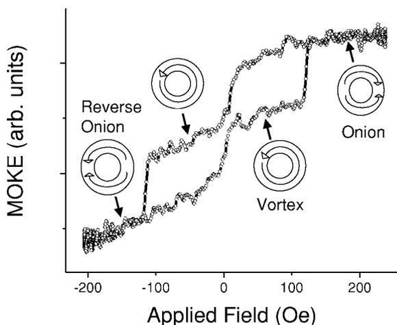
FIG. 1. Hysteresis loop from a single 5  $\mu\text{m}$  diameter permalloy ring. Schematic diagrams indicating the magnetic states of the ring are also shown.
