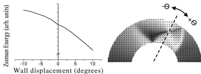
FIG. 4. Simulated variation of Zeeman energy with wall displacement in a  $1 \mu\text{m}$  diameter permalloy ring.
