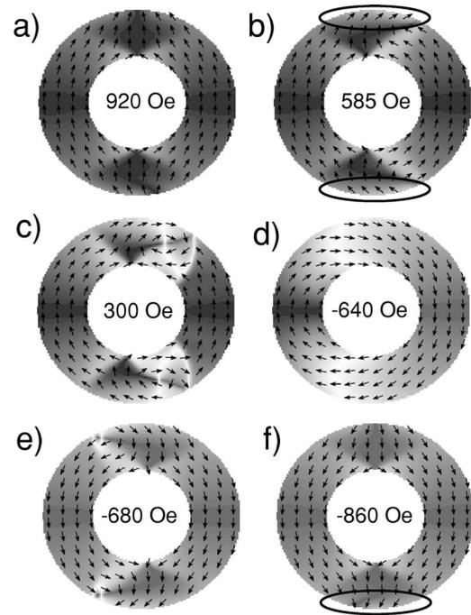
FIG. 3. Magnetic configurations from a micromagnetic simulation of a  $1\ \mu\text{m}$  diameter permalloy ring with a width of  $0.25\ \mu\text{m}$  and a thickness of  $45\ \text{nm}$ .
