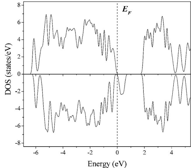
FIG. 3. Density of states of  $\text{Ti}_3\text{CuO}_7$ , with the oxygen vacancy near Cu. Positive values are for spin up and the negative ones for spin down. Energies are referred to the Fermi level,  $E_F$ . The minority spin feature inside the gap but close to  $E_F$  is 50% of Cu 3d and 50% of oxygen and Ti character.
