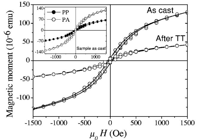
FIG. 2. Room-temperature hysteresis curve of the Cu-doped  $\text{TiO}_{2-\delta}$  film (points) in the sample as cast and after a thermal treatment (TT) at 800 °C for 30 min in a oxygen-rich atmosphere. Solid lines are the best least-squares fits of Eq. (1) to the data. The inset compares the hysteresis loops measured with the external magnetic field applied parallel (PA) and perpendicular (PP) to the film plane for the as cast sample.
