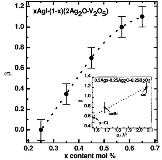
FIG. 3. Plot of the variation of the exponent  $\beta$  with different amount of AgI content in  $\text{AgI} \cdot (1-x)(2\text{Ag}_2\text{O} \cdot \text{V}_2\text{O}_5)$  glasses. Inset shows the variation of the exponent  $\beta$  vs the average electronic polarizability per atom/ion,  $\alpha$ , in  $0.5\text{AgX} \cdot 0.25\text{Ag}_2\text{O} \cdot 0.25\text{B}_2\text{O}_3$  glasses. The dashed lines are drawn as guides to the eye.
