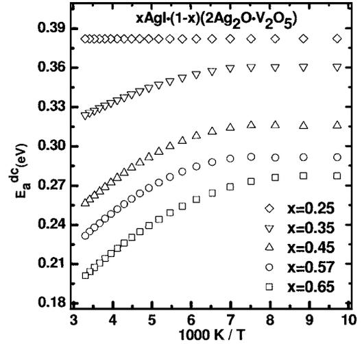
FIG. 2. The variation of the “apparent activation energy” with temperature in  $x\text{AgI}\cdot(1-x)(2\text{Ag}_2\text{O}\cdot\text{V}_2\text{O}_5)$  with  $0.25 \leq x \leq 0.65$  glasses.
