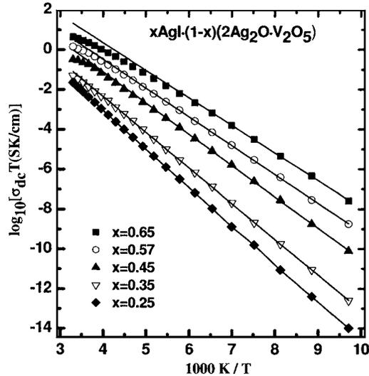
FIG. 1. Arrhenius plot of the dc conductivity (multiplied by the temperature) of  $x\text{AgI}\cdot(1-x)(2\text{Ag}_2\text{O}\cdot\text{V}_2\text{O}_5)$  with  $0.25 \leq x \leq 0.65$  glasses. The symbol represents the experimental data points and the fitted line corresponds to using the Arrhenius law.
