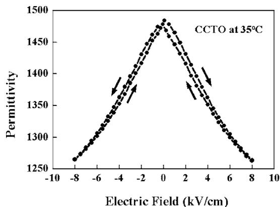
FIG. 4. Dependence of the dielectric constant of CCTO on bias electric field at 35 °C (at 10 kHz).
