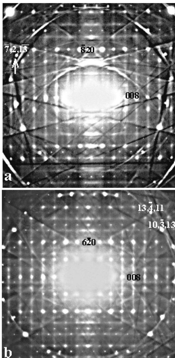
FIG. 3. Typical (a)  $\langle 140 \rangle$  and (b)  $\langle 130 \rangle$  zone axis EDPs of CCTO. Note the characteristic transverse polarized diffuse streaking running perpendicular to the  $\langle 001 \rangle^*$  directions of reciprocal space.
