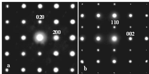
FIG. 2. Typical (a)  $\langle 001 \rangle$  and (b)  $\langle 110 \rangle$  zone axis EDPs of CCTO.
