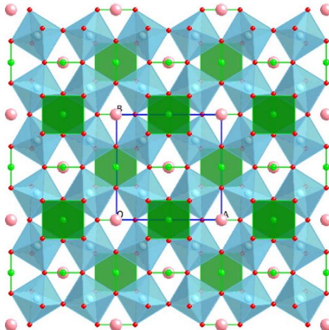
FIG. 1. (Color online) The  $Im\bar{3}$  average crystal structure of  $\text{CaCu}_3\text{Ti}_4\text{O}_{12}$  in projection along  $\langle 001 \rangle$  showing the tilted  $\text{TiO}_6$  octahedral network as well as the  $\text{CuO}_4$  square planar coordination of the Cu ions.
