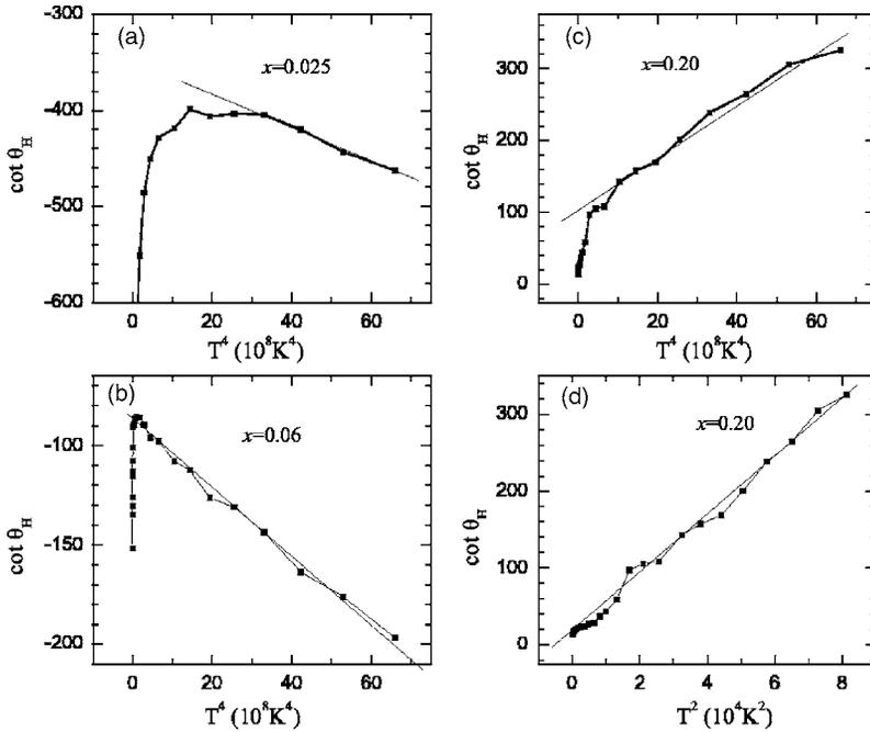
FIG. 3. Temperature dependence of  $\cot \theta_H (\sim \rho_{ab}/R_H)$  at 10 T in  $T^4$  scale for the crystals  $\text{Nd}_{2-x}\text{Ce}_x\text{CuO}_4$ . (a)  $x=0.025$ , (b)  $x=0.06$ , (c)  $x=0.20$ , and (d)  $x=0.20$  in  $T^2$  scale.
