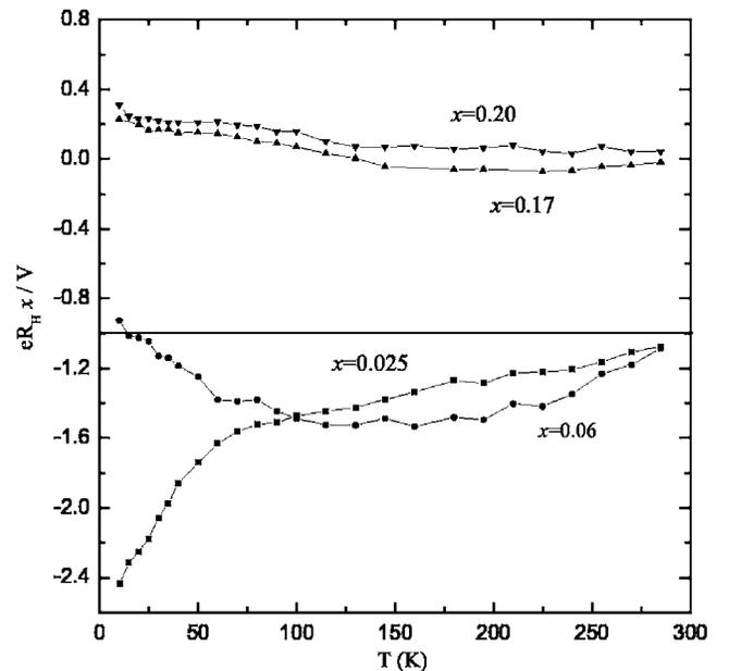
FIG. 4.  $eR_Hx/V$  as a function of temperature for the  $\text{Nd}_{2-x}\text{Ce}_x\text{CuO}_4$  crystals with  $x=0.025$ ,  $0.06$ ,  $0.17$ , and  $0.20$ .
