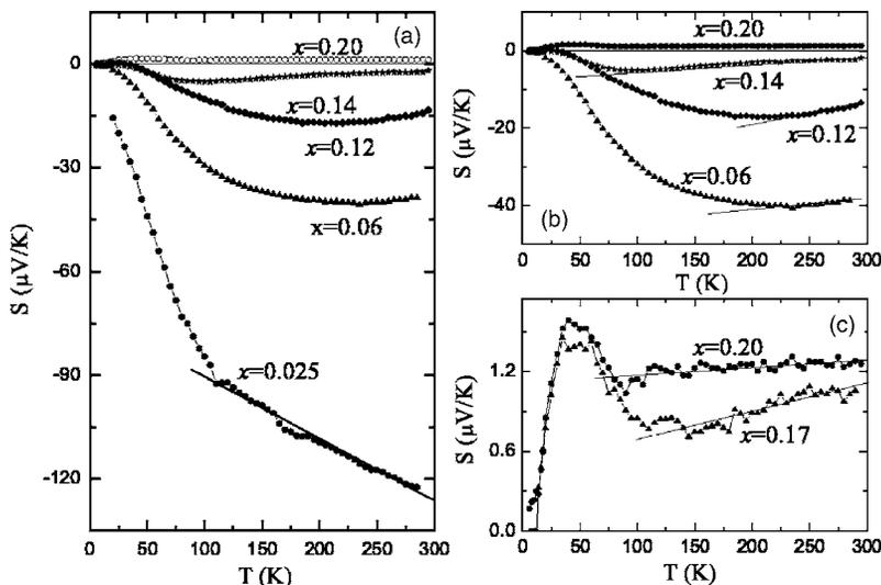
FIG. 2. (a) Temperature dependence of thermoelectric power (TEP) for the Nd<sub>2-x</sub>Ce<sub>x</sub>CuO<sub>4</sub> crystals with different doping levels. (b) TEP vs T for  $x=0.06$ , 0.12, 0.14, 0.20. (c) TEP vs T for the overdoped samples.
