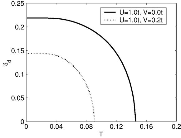
FIG. 1. Variation of the CDW order parameter  $\delta_d$  with temperature in the absence (solid line) and presence (dotted line) of an on-site hybridization potential.
