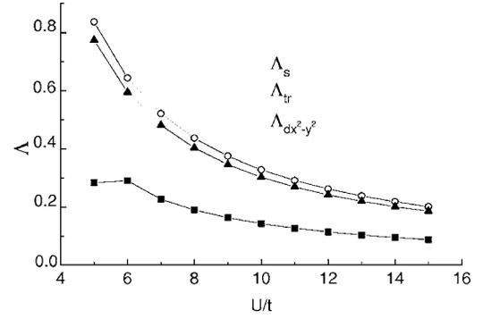
FIG. 7. Renormalization constants  $\Lambda_\alpha$  for different pairing channels and for transport  $\Lambda_t$  relevant for transport for the Hubbard model with  $t' = 0$  at increasing  $U$ . The temperature is fixed at  $\beta = 50/t$ , the doping at  $\delta = 0.12$ .
