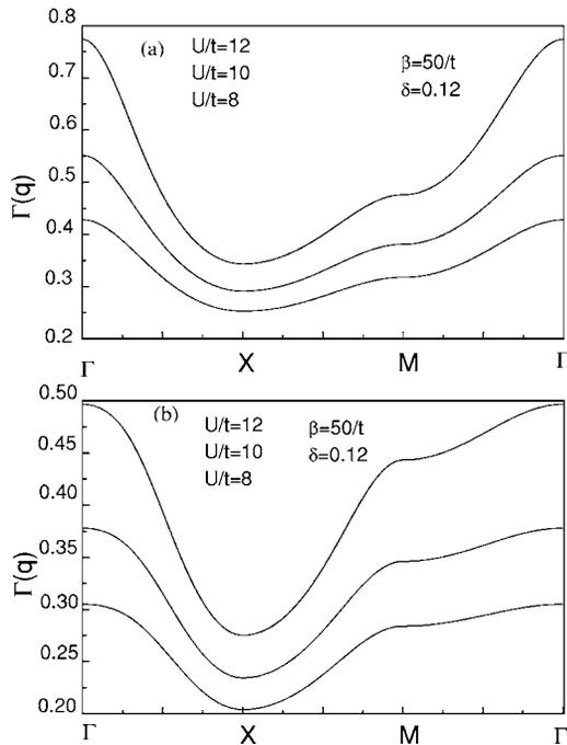
FIG. 4. The electron-phonon vertex  $\Gamma(q)$  for scattering electrons on the Fermi surface. Calculations are for the Hubbard model with  $t'=0$  (a) and  $t'=-0.35t$  (b), the values of the Coulomb interaction are  $U/t=12, 10, 8$  from above. The temperature is fixed at  $\beta=50/t$ , the doping at  $\delta=0.12$ .
