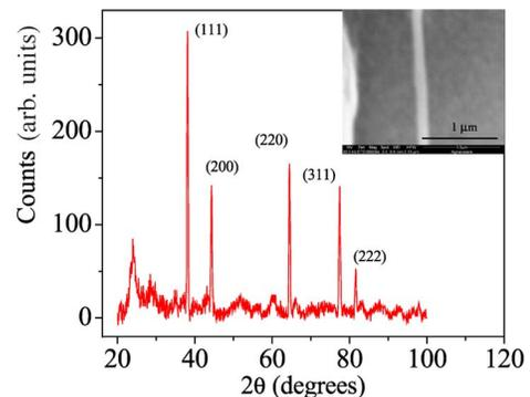
FIG. 1. (Color online) XRD of the 15 nm Ag nanowires. The inset shows the SEM image of a 100 nm wire.
