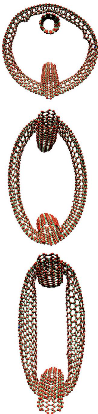
FIG. 10. (Color online) Tensile loading of nanoring without side constraints.
