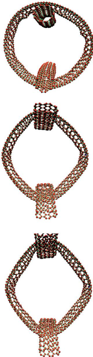
FIG. 13. (Color online) Tensile loading of nanoring with side constraints.
