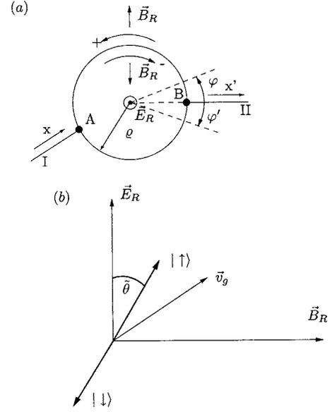
FIG. 1. (a) Momentum-dependent in-plane Rashba field  $\vec{B}_R$ , and (b) up and down spin eigenstates do not generally align with the Rashba field  $\vec{B}_R$ , but make a tilt angle  $\theta$  with the electric field  $\vec{E}_R$  perpendicular to the ring plane ( $\vec{E}_R$ ,  $\vec{B}_R$ , and  $\vec{v}_g$  form an orthogonal coordinate system).
