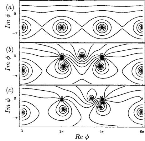
FIG. 3. Zero-pole structure of  $G$  in the complex plane for  $\beta=0$  and (a)  $R=1$ , (b)  $R=1/2$ , (c)  $R\approx 0.55$ . The zeros lie on the real axis, whereas the poles have a finite imaginary part.
