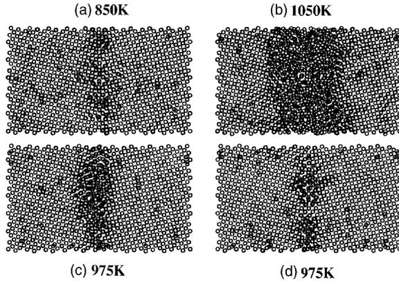
FIG. 3. The configuration of GB at high temperature. (a) The GB structure at 850 K (high-temperature disordered state). (b) The GB structure at 1050 K (melting state). (c) and (d) The GB structure at 975 K (superheated state) with unstable liquid film.
