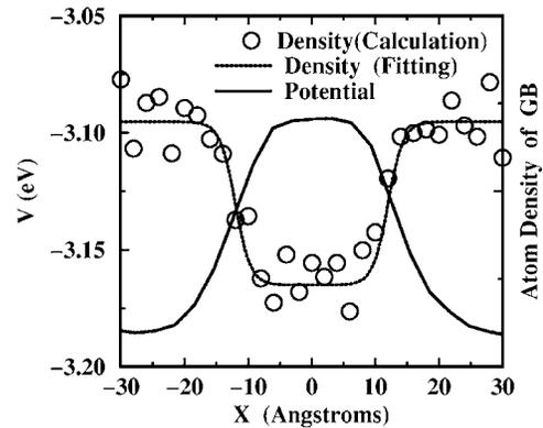
FIG. 5. The profile of potential and atomic density across the GB at 975 K.
