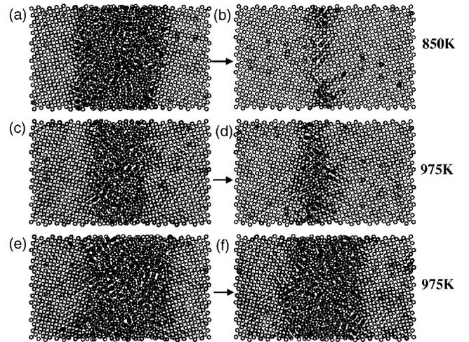
FIG. 4. The response of superheated state for adding liquid film. (a) and (b) at 850 K,  $2l = 30 \text{ \AA}$ . (c) and (d) at 975 K,  $2l = 20 \text{ \AA}$ . (e) and (f) at 975 K,  $2l = 30 \text{ \AA}$ .
