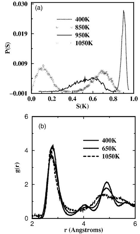
FIG. 2. The distribution functions  $P(S)$  (a) and the pair-correlation functions (b) at various temperatures. The flat and wide distribution of  $S(\mathbf{K})$  at 950 K represents the coexistence of liquid and solid.
