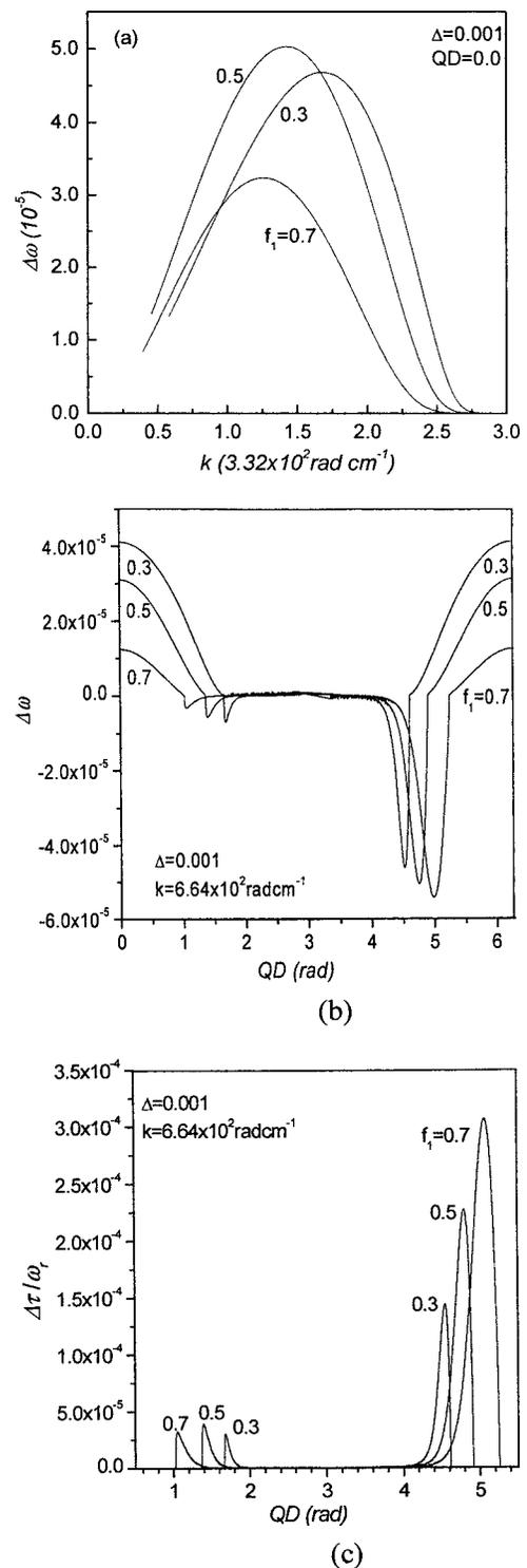
FIG. 4. Nonlinear shift in frequency and attenuation of modes in the top band. (a) shows the shift as a function of  $k$  for various thicknesses of magnetic layers  $f_1$ . (b) indicates the shift versus  $QD$  for a fixed  $k$  and different  $f_1$  and (c) illustrates the nonlinear attenuation as a function of  $QD$  with  $k$  and  $f_1$  as the same as those in (b).
