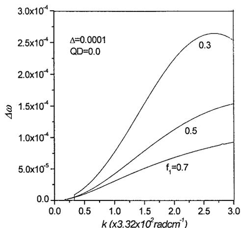
FIG. 5. Nonlinear frequency shift  $\Delta\omega$  of the modes in the middle band versus  $k$  for  $QD=0$ ,  $\Delta=1.0\times 10^{-4}$  and various values of  $f_1$ .
