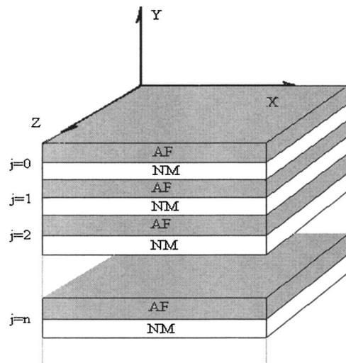
FIG. 1. Geometry and coordinate system. The superlattice is composed of antiferromagnetic layers (AFs) with thickness  $d_1$  and nonmagnetic layers (NMs) with thickness  $d_2$ . The two sublattice magnetizations in AF layers are parallel and antiparallel to the  $z$  axis, respectively. The  $y$ -axis is pointed normal to the interfaces and the polariton waves propagate along the  $x$ -axis for the surface modes and in the  $x$ - $y$  plane for the bulk modes.  $j$  is the index of supercell.
