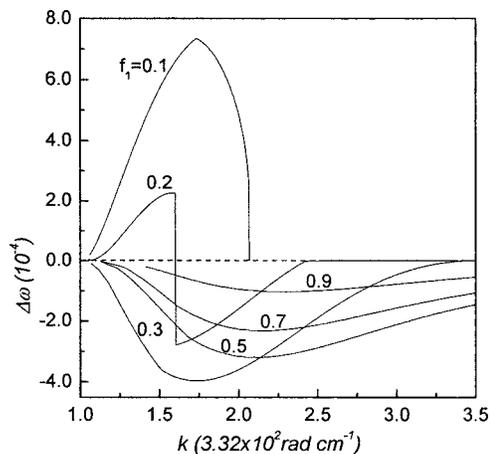
FIG. 6. Nonlinear frequency shift  $\Delta\omega$  of the surface mode versus  $k$  for  $\Delta=1.0\times 10^{-4}$  and various values of  $f_1$ .
