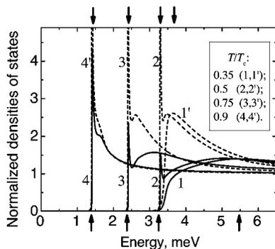
FIG. 2. The temperature effect on the normalized densities of states  $N_i(E)/N_i(0)$ . Curves 1–4 and 1'–4' are the data for larger-gap and smaller-gap groups, respectively. Arrows below and above the figure show the main peak positions in the  $N_1(E)$  and  $N_2(E)$  characteristics. The calculations have been done for the parameters indicated in the caption to Fig. 1.
