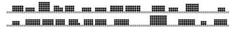
FIG. 1. Typical atomic configuration at the end of the simulation ( t = 10^{14} of inverse hopping rate units) at the coverage \theta = 2 . Black squares, the deposited atoms; gray squares, those of the substrate. A small portion of the simulated system of about 16 000 sites was chosen randomly with the only bias that the whole islands were visible.
