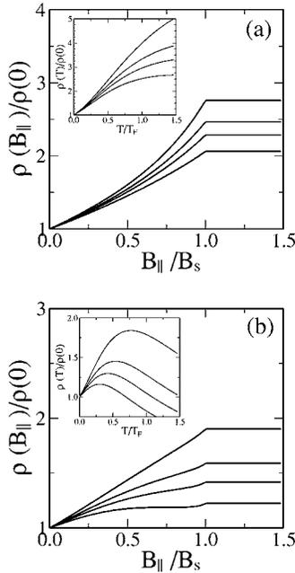
FIG. 2. The calculated  $\rho(B_{\parallel})$  in  $n$ -GaAs (a) for ideal 2D system and (b) for quasi-2D system at  $T=0$  and for various densities  $n=0.4, 0.8, 1.2, 2.0 \times 10^{10} \text{ cm}^{-2}$ , (from top to bottom). The insets show  $\rho(T)$  at  $B_{\parallel}=0$  and for the same systems as the main figures.
