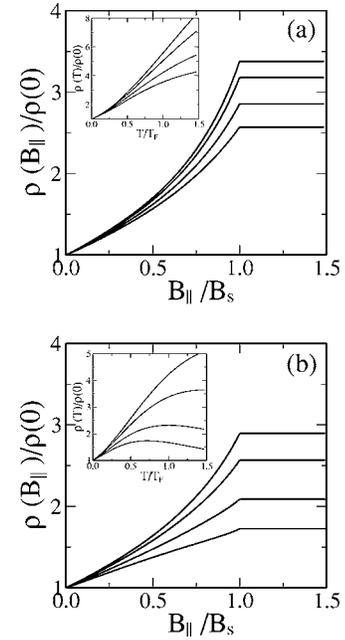
FIG. 1. The calculated  $\rho(B_{\parallel})$  in Si MOSFETs (a) for ideal 2D system and (b) for quasi-2D system at  $T=0$  and for various densities  $n=1.0, 2.0, 5.0, 10.0 \times 10^{11} \text{ cm}^{-2}$  (from top to bottom). The insets show  $\rho(T)$  at  $B_{\parallel}=0$  and for the same systems as the main figures.
