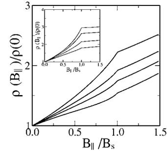
FIG. 4. The main figure (inset) shows the calculated  $\rho(B_{\parallel})$  in the realistic quasi-2D  $n$ -GaAs (Si MOS) system including both magneto-spin-polarization and magneto-orbital effects for various densities  $n=0.4, 0.8, 1.2, 2.0 \times 10^{10} \text{ cm}^{-2}$  ( $n=1.0, 2.0, 5.0, 10.0 \times 10^{11} \text{ cm}^{-2}$ ), from top to bottom.
