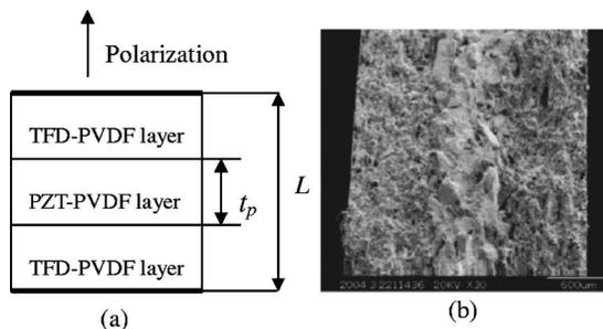
FIG. 1. (a) Schematic illustration and (b) a typical micrograph of the fractured surface of the laminated *TPT* composites. TFD denotes Terfenol-*D*.
