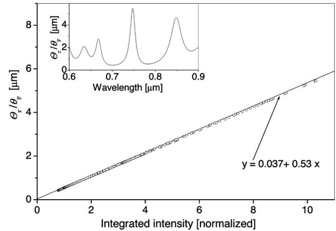
FIG. 5. FRR [ $\Theta_r(\lambda)$ ] normalized to the bulk rotation per  $\mu\text{m}$  [ $\theta_F(\lambda)$ ] as a function of the integrated intensity [see RHS of Eq. (2)]. Note that the straight line is identical to the straight line in Fig. 4. The inset shows  $\Theta_r(\lambda)$  vs wavelength.
