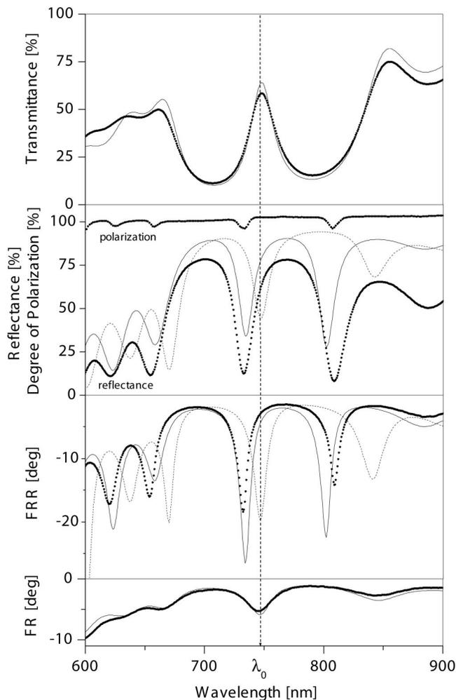
FIG. 2. Spectra of transmittance, reflectance, Faraday rotation in reflection (FRR), Faraday rotation in transmission (FR), and the degree of polarization of the BIG-YIG MPC. Symbols represent measured data, solid lines represent calculated spectra of the MPC, and dashed lines represent spectra calculated for a MPC where the thickness of the top BIG layer has been increased by 64%. Measurements and calculations of reflectance and FRR were performed on the MPC covered by a silver layer.
