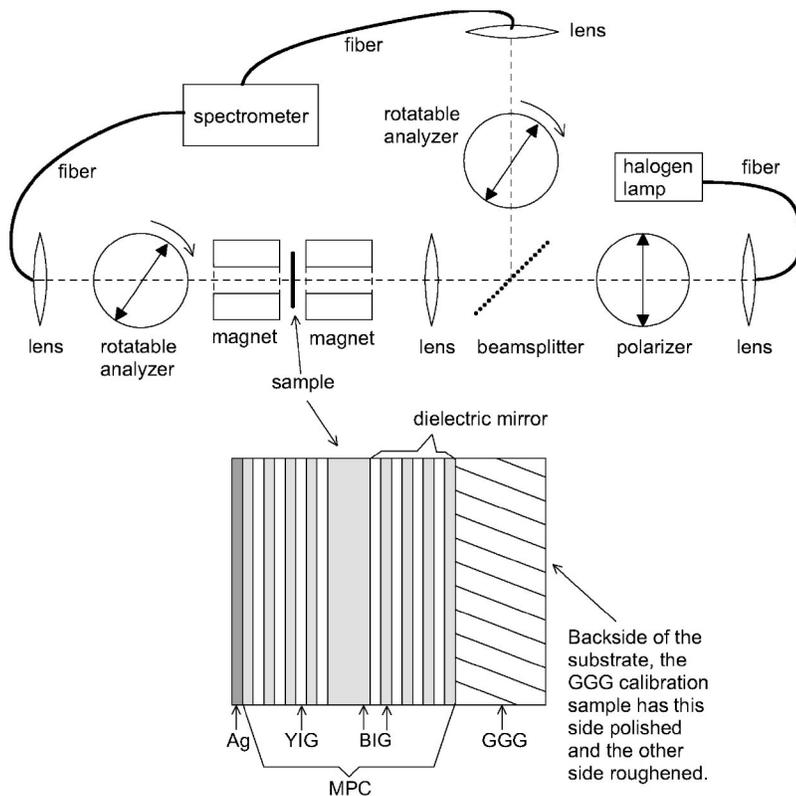
FIG. 1. Setup for measurement of transmittance, reflectance, and Faraday rotation of transmitted and reflected light. The position of the rotatable analyzer depends on whether the measurement is performed in transmission or reflection.
