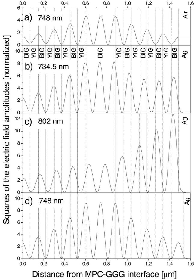
FIG. 3. Calculated intensity distributions inside BIG-YIG MPCs. (a) MPC without silver cover at resonance. (b) MPC covered with silver layer at the first resonance. (c) MPC with silver cover at the second resonance. (d) MPC with silver cover and compensation for phase shift at resonance.
