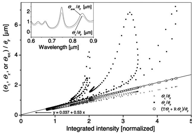
FIG. 4. Calculated FR [ $\Theta_t(\lambda)$ ], FRR [ $\Theta_r(\lambda)$ ], and averaged MO rotation [ $\Theta_{\text{ave}}(\lambda)$ ] normalized to the bulk rotation per  $\mu\text{m}$  [ $\theta_F(\lambda)$ ] as a function of the integrated intensity [see RHS of Eq. (2)]. The inset shows  $\Theta_t(\lambda)/\theta_F(\lambda)$  and  $\Theta_{\text{ave}}(\lambda)/\theta_F(\lambda)$  vs wavelength.
