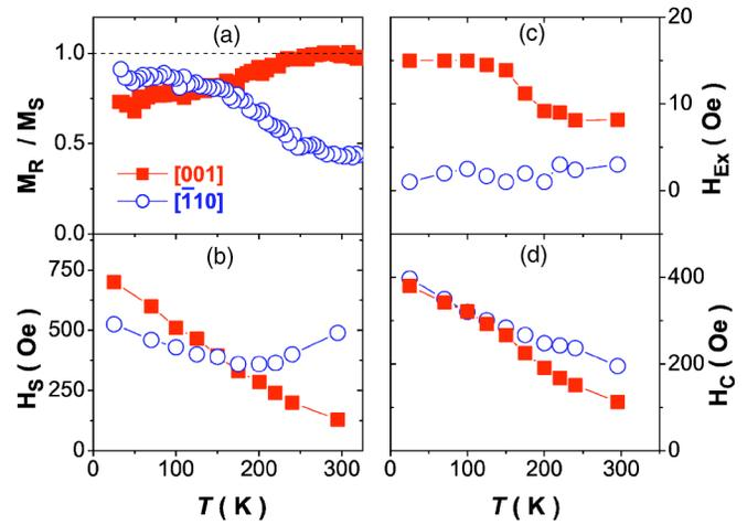
FIG. 3.  $\text{Ni}_{81}\text{Fe}_{19}$  on  $(11\bar{2}0)$   $\alpha\text{-Fe}_2\text{O}_3$ : temperature dependence of (a) normalized remanent magnetization ( $M_r/M_s$ ), (b) saturation field ( $H_s$ ), (c) the  $H_{\text{Ex}}$ , and (d) the  $H_C$  with the in-plane direction.
