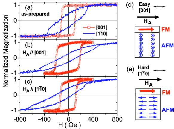
FIG. 4. The room-temperature magnetic hysteresis loops of  $\text{Ni}_{81}\text{Fe}_{19}$  on  $(11\bar{2}0)$   $\alpha\text{-Fe}_2\text{O}_3$  (a) without MFA, (b) with MFA perpendicular to the AF spin direction, and (c) with MFA parallel to the AF spin direction. Two schematic MFA configurations were also displayed in (d) and (e). Here,  $H_A$  means the annealing magnetic field.
