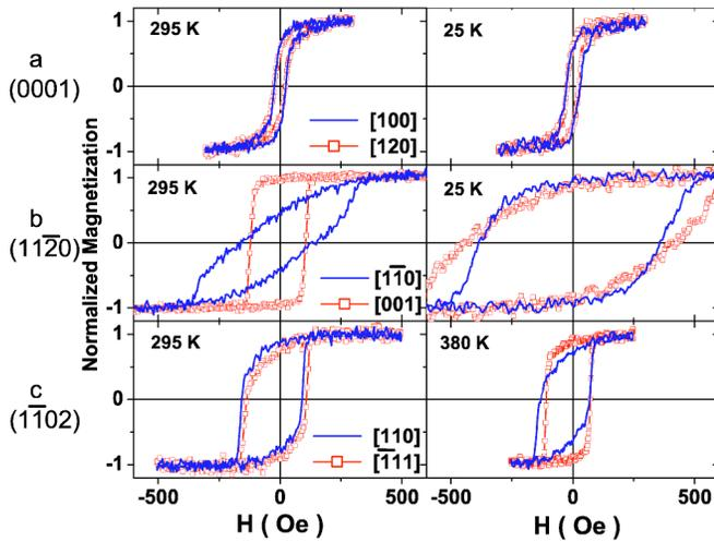
FIG. 1. The magnetic hysteresis loops of as-prepared  $\text{Ni}_{81}\text{Fe}_{19}$  on (a) (0001)  $\alpha\text{-Fe}_2\text{O}_3$ , (b)  $(11\bar{2}0)$   $\alpha\text{-Fe}_2\text{O}_3$ , and (c)  $(1\bar{1}02)$   $\alpha\text{-Fe}_2\text{O}_3$  at several temperatures.
