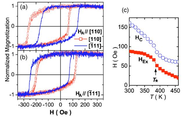
FIG. 5. The room-temperature magnetic hysteresis loops of  $\text{Ni}_{81}\text{Fe}_{19}$  on  $(1\bar{1}02)$   $\alpha\text{-Fe}_2\text{O}_3$  (a) with MFA along the  $[110]$  direction and (b) with MFA along the  $[\bar{1}11]$  direction. The temperature-dependent  $H_{\text{Ex}}$  and  $H_C$  was displayed in (c). The  $T_*$  roughly agrees with the Morin temperature of  $(1\bar{1}02)$   $\alpha\text{-Fe}_2\text{O}_3$ .
