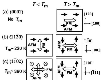
FIG. 2. Schematic surface spin structures of  $\alpha\text{-Fe}_2\text{O}_3$  on (a) (0001)  $\alpha\text{-Al}_2\text{O}_3$ , (b)  $(11\bar{2}0)$   $\alpha\text{-Al}_2\text{O}_3$ , and (c)  $(1\bar{1}02)$   $\alpha\text{-Al}_2\text{O}_3$ .
