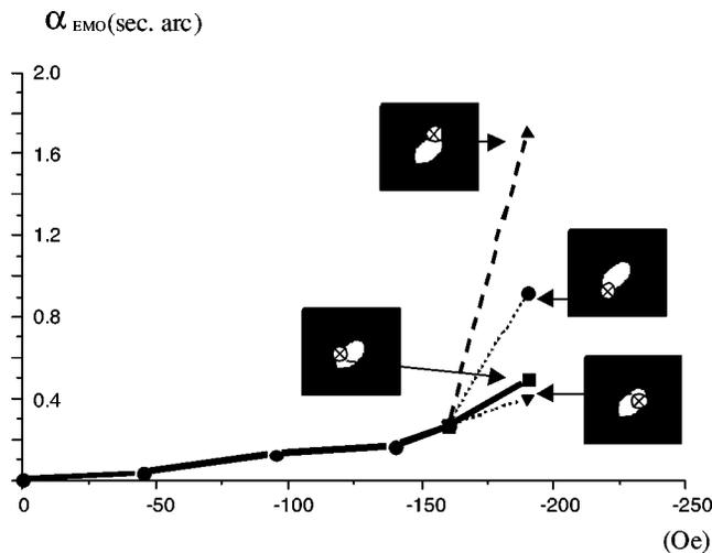
FIG. 4. The changes of the magnetic-field dependencies of EMOE for the different sites of a domain wall in the magnetic fields close to the domain collapse.
