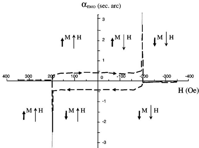
FIG. 2. The magnetic-field dependence of EMOE in a full cycle of the domain remagnetization (qualitative picture). The arrows on the curves show the path-tracing direction of the magnetic field changing. The sketches on the figure show the mutual orientations of  $\mathbf{M}$  and  $\mathbf{H}$  vectors for the different magnetic-field regions.
