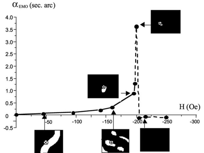
FIG. 3. The magnetic-field dependence of the EMOE measured on the film region with a domain wall in the different stage of the domain decreasing up to the full collapsing.
