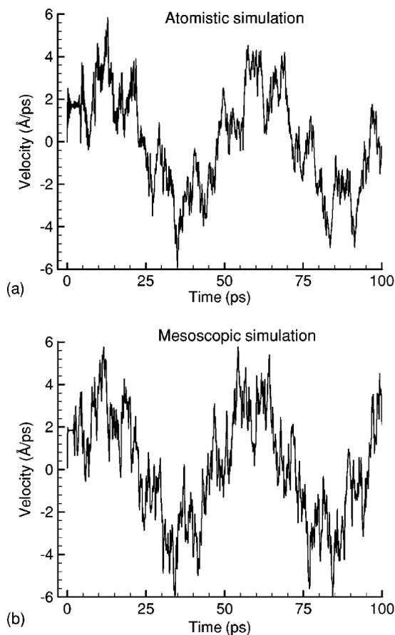
FIG. 7. Velocity of an end part of a 395 Å long (10,10) CNT in atomistic (a) and mesoscopic (b) simulations of free bending vibrations, illustrated in Fig. 6. In the atomistic simulation, the velocity is averaged over atoms that belong to a  $\sim 1$  nm long end segment of the CNT, in the mesoscopic simulation the velocity of an end node is plotted.
