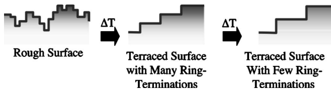
FIG. 7. Schematic depiction of the proposed model for evolution of long-range surface morphology at 700–950 K.
