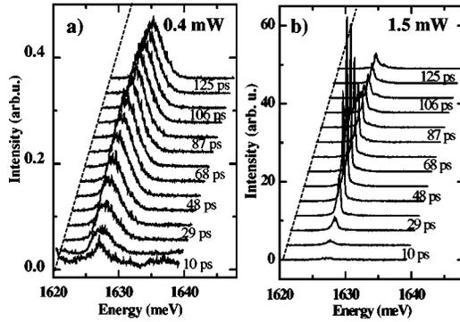
FIG. 1. PL spectra at  $k_{\parallel}=0$  measured at different time delays after the excitation pulse for (a)  $P=0.4$  mW and (b)  $P=1.5$  mW. Spectra have been vertically and horizontally shifted for clarity. Vertical arbitrary units in (a) and (b) are the same.
