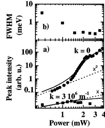
FIG. 3. (a) Circles (squares): peak intensity measured for  $k_{\parallel}=0$  ( $k_{\parallel}=310^6$  m<sup>-1</sup>) as a function of the excitation power. Solid lines: calculated peak intensities as a function of the excitation power for  $k_{\parallel}=0$  and  $k_{\parallel}=3 \times 10^6$  m<sup>-1</sup>. (b) Spectral full width at half maximum measured in  $k_{\parallel}=0$  at the time delay corresponding to the peak intensity.
