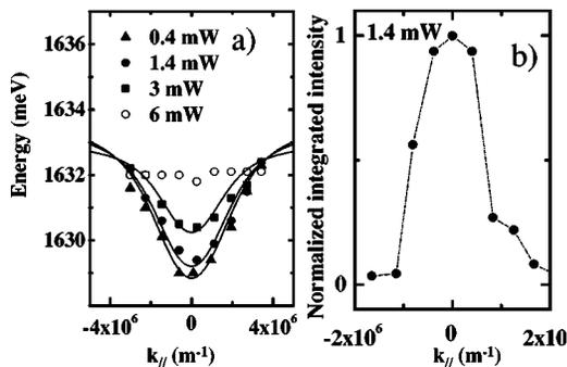
FIG. 2. (a) Symbols: PL peak energy measured at short time delays (20 ps after the laser pulse) as a function of  $k_{\parallel}$  for various excitation powers. Solid lines: calculated dispersion relations with a Rabi splitting of 10.5, 9.5, and 6.7 meV. (b) Integrated intensity measured as a function of  $k_{\parallel}$  for a 1.4 mW excitation power.
