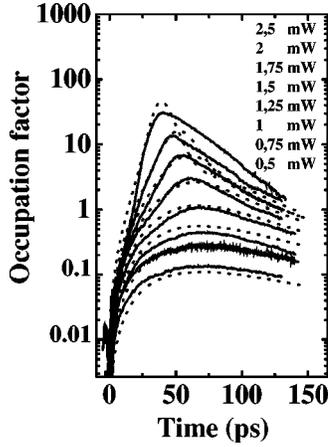
FIG. 4. Solid lines: occupation factor measured at  $k_{\parallel}=0$  as a function of time for various excitation powers. Dashed lines: calculated occupation factors as a function of time for the same excitation conditions. The laser arrival time lies close to  $t=0$ .
