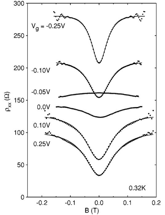
FIG. 5. Examples of the experimental, semiclassical resistivity  $\rho_{xx}^{sc}$  at various fixed gate voltages  $V_g$  as a function of the magnetic field  $B$  at 0.32 K. The filled circles are the measured values and the lines are fitted curves using Eqs. (2) and (3). The experimental data have been smoothed to reduce the deHS oscillations (as explained in the text).
