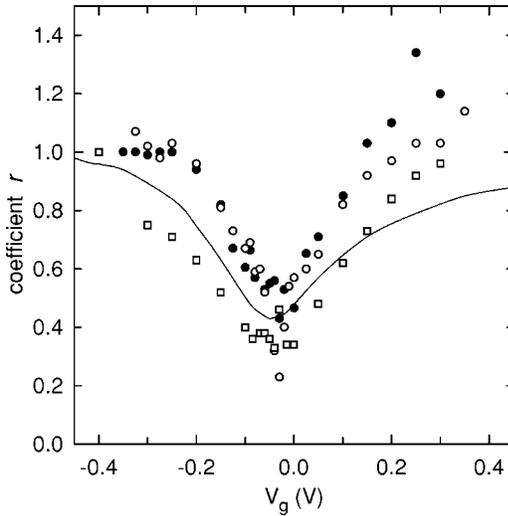
FIG. 6. The coefficient  $r$  in Eq. (2) as a function of gate voltage  $V_g$ . The symbols are experimental data: open circles are 0.32 K, filled circles are 1.09 K, and open squares are 4.2 K. The line was calculated by using Eq. (17), as explained in the text.
