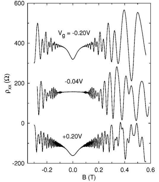
FIG. 2. Examples of data on the resistivity  $\rho_{xx}$ , at 0.32 K as a function of magnetic field  $B$  at various fixed gate voltages  $V_g$ . The top curve is offset by  $+150 \text{ } \Omega$  and the bottom by  $-200 \text{ } \Omega$ .
