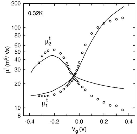
FIG. 7. The transport mobilities  $\mu^t$  as a function of gate voltage  $V_g$ . The open circles are the measured quantities at 0.32 K evaluated from the semiclassical magnetoresistivities. The lines were calculated by using Eqs. (7)–(15), as described in the text.
