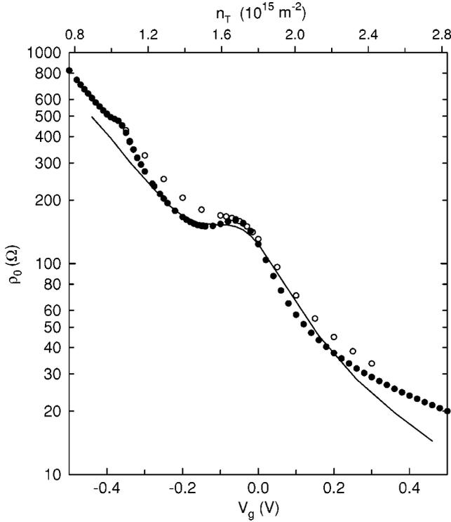
FIG. 1. The zero-field resistivity,  $\rho_0$ , as a function of gate voltage  $V_g$  and total carrier concentration  $n_T$ . The resonance is near  $V_g = -0.04$  V. The filled and open circles are data at 0.32 K and 4.2 K, respectively. The line was calculated using the model described in the text.
