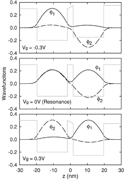
FIG. 10. Examples of calculated wave functions in the DQW at three fixed gate voltages  $V_g$ . The solid lines correspond to the symmetric state and the dashed lines to the antisymmetric state. The locations of the two wells (and their relative depths, not to scale) are indicated by gray lines.
