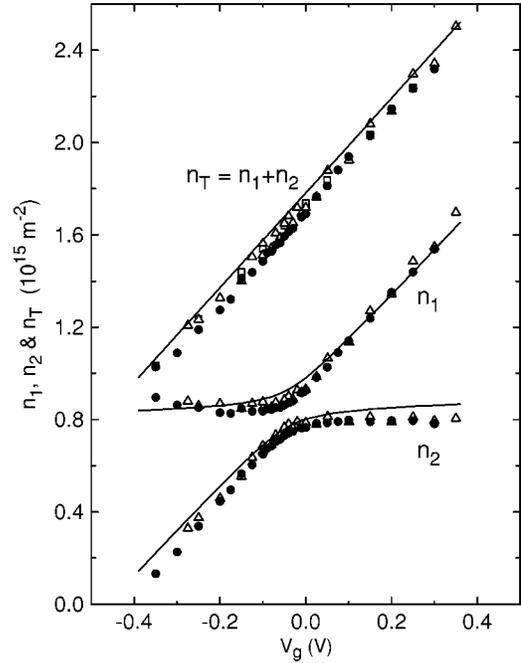
FIG. 3. The carrier densities as functions of gate voltage  $V_g$ . The filled circles and open triangles are results evaluated from the deHS data at 0.32 K and 1.09 K, respectively. The open squares are from the Hall data at 1.10 K. The lines were calculated using the model described in the text.
