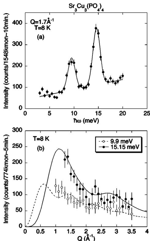
FIG. 6. (a) Constant- $Q$  scans at 8 K in  $Sr_3Cu_3(PO_4)_4$ . The solid line is the result of a fit with two Gaussians. (b)  $Q$  dependence of neutron-scattering intensity at 9.9 meV and 15.15 meV. Background intensity measured at a different energy is subtracted from the raw data. The lines show the intensity calculated using Eq. (3).
