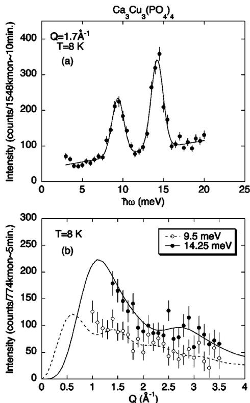
FIG. 5. (a) Constant- $Q$  scans at 8 K in  $Ca_3Cu_3(PO_4)_4$ . The solid line is the result of a fit with two Gaussians. (b)  $Q$  dependence of neutron-scattering intensity at 9.5 meV and 14.25 meV. Background intensity measured at a different energy is subtracted from the raw data. The lines show the intensity calculated using Eq. (3).
