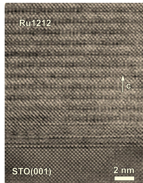
FIG. 3. Cross-section HREM image of a Ru-1212 island (Fig. 2(a)). The film is c oriented.
