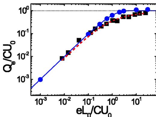
FIG. 4. (Color online) Normalized extracted charge as a function of normalized number of photogenerated charge carriers. The squares are the experimentally measured values, circles are the calculated data, using the full numerical model, while the full line is the fit, using Eq. (6). The dashed line is calculated including exciton bimolecular annihilation (see text). The dotted line shows when the extracted charge equals  $CU_0$ .
