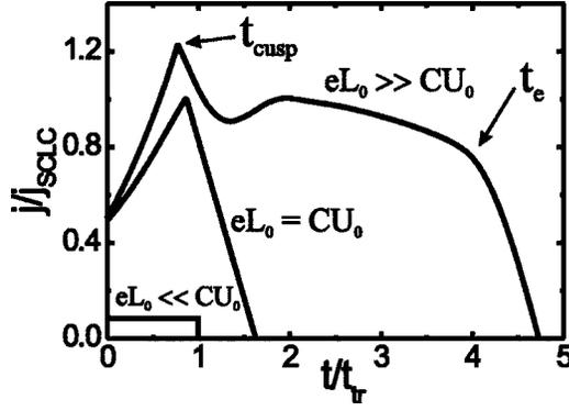
FIG. 1. Schematic current transients ( $j$ -TOF) as a function of light intensity with no carrier recombination.
