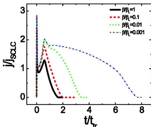
FIG. 3. (Color online) Numerically calculated current transients for various  $\beta/\beta_L$  ratios. The parameters used in calculations are  $R'=0.004$ ,  $\alpha d=35$  with the normalized number of photogenerated charge carriers  $L'_0=30$ . Please note the similarities to Fig. 1 which shows transients without recombination.
