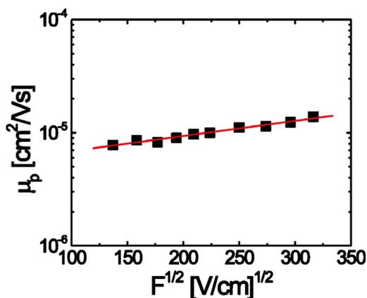
FIG. 5. (Color online) Experimentally measured hole mobility as a function of electric field for RRaPHT.
