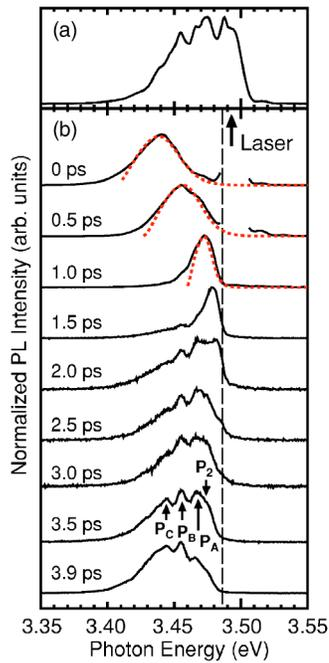
FIG. 4. (Color online) Temporal changes of PL spectra of GaN thin films under the  $A$ -exciton resonant excitation (3.493 eV). The excitation density is  $330 \mu\text{J}/\text{cm}^2$ . Time-integrated PL spectra are shown in (a). The broken curves are fitting using a non- $k$ -conservation model.
