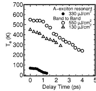
FIG. 5. Effective electron temperature ( $T_e$ ) as a function of the delay time. Open circles and triangles are under the band-to-band excitation, and solid circles are under the  $A$ -exciton resonant excitation. The excitation intensity is shown in the figure.
