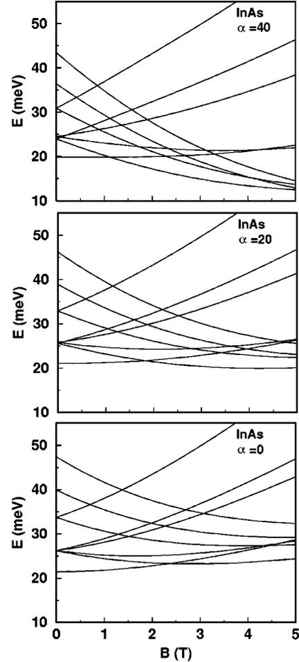
FIG. 1. Energy spectrum of a two-electron InAs quantum dot versus the applied magnetic field for different values of the Bychkov-Rashba interaction parameter  $\alpha$  (meV nm). For clarity, at each value of the magnetic field and for a given total angular momentum, only the lowest energy is plotted. The Zeeman angular is also included.
